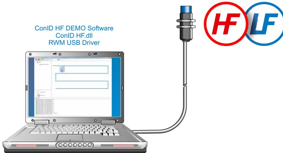
The default address of USB Read/Write Modules is 254.
