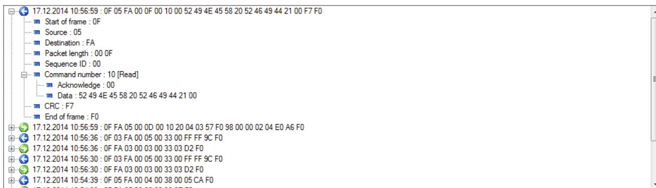
This tool is extremely useful because it shows the structure of exchanged frames and provides full information to the integrator during programming of the controller or PLC that controls the industrial bus.
